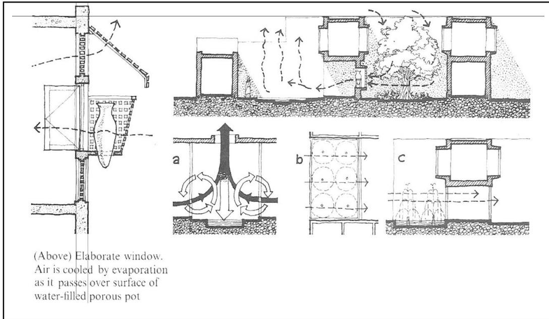
Figure 2. Evaporative coolers in front of window hoods in arid climate and wind convection over interior water pools. Source: Konya, A. Design Primer for Hot Climates, London: The Architectural Press Ltd. 1984.
