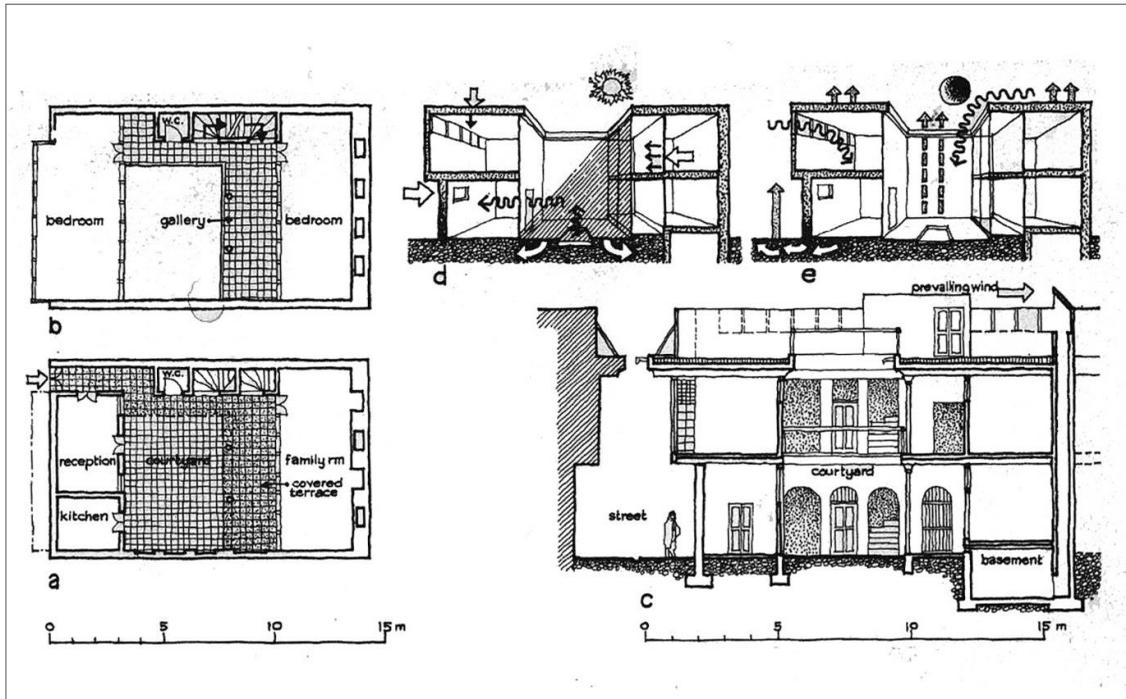
Figure 3. Enclosed Courtyards and Wind Towers as means of cooling the house interiors in arid regions. Source: Konya, A (1984) Design Primer for Hot Climates. London, The Architectural Press Ltd.
